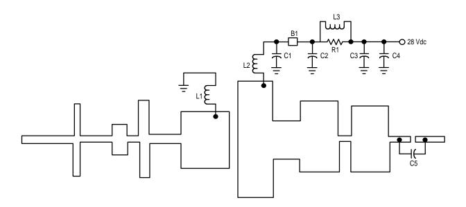
Board Material – Teflon<sup>®</sup> Glass Laminate Dielectric Thickness = 0.30",  $\epsilon_{\text{f}}$  = 2.55", 2.0 oz. Copper
