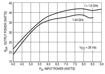
Figure 3. Output Power versus Input Power
