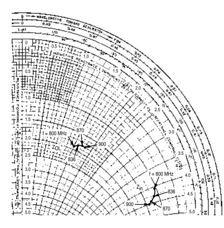
$P_{out}$  = 20 W,  $V_{CC}$  = 12.5 Vdc
