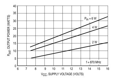
Figure 4. Output Power versus Supply Voltage
