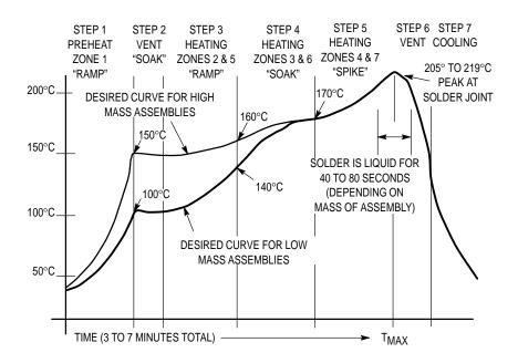
Figure 1. Typical Solder Heating Profile
