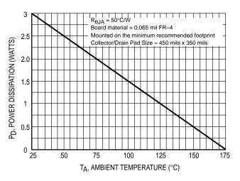
Figure 15. D<sup>2</sup>PAK Power Derating Curve
