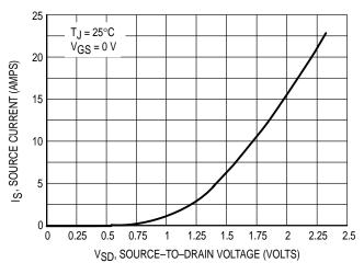
Figure 10. Diode Forward Voltage versus Current
