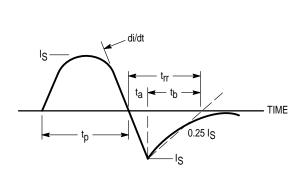
Figure 14. Diode Reverse Recovery Waveform
