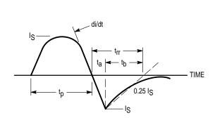
Figure 14. Diode Reverse Recovery Waveform
