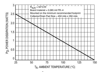
Figure 15. D<sup>2</sup>PAK Power Derating Curve
