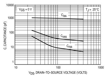
Figure 7b. High Voltage Capacitance Variation
