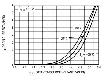
Figure 2. Transfer Characteristics
