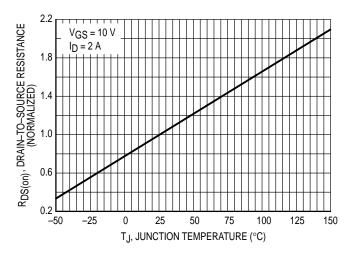
Figure 5. On–Resistance Variation with Temperature
