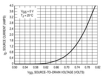
Figure 10. Diode Forward Voltage versus Current
