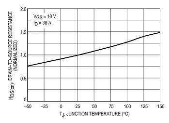
Figure 5. On–Resistance Variation with Temperature
