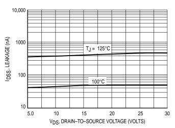
Figure 6. Drain-To-Source Leakage Current versus Voltage
