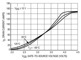
Figure 2. Transfer Characteristics
