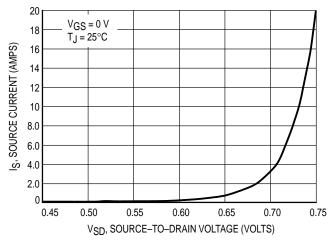
Figure 10. Diode Forward Voltage versus Current
