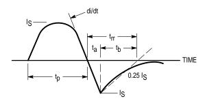
Figure 15. Diode Reverse Recovery Waveform
