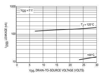
Figure 6. Drain-to-Source Leakage Current versus Voltage
