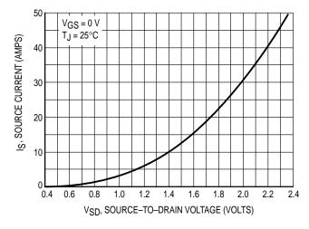
Figure 10. Diode Forward Voltage versus Current
