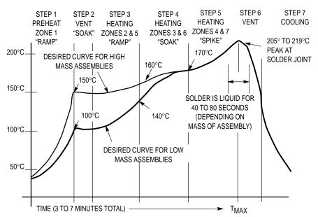
Figure 19. Typical Solder Heating Profile
