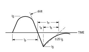
Figure 15. Diode Reverse Recovery Waveform
