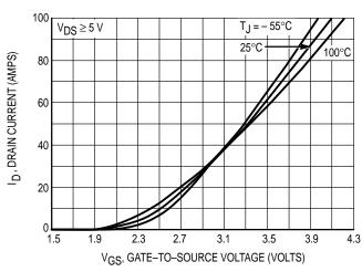
Figure 2. Transfer Characteristics
