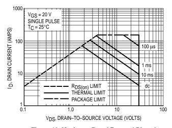
Figure 12. Maximum Rated Forward Biased Safe Operating Area
