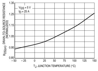
Figure 5. On–Resistance Variation with Temperature
