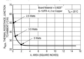
Figure 17. Thermal Resistance versus Drain Pad Area for the D<sup>2</sup>PAK Package (Typical)
