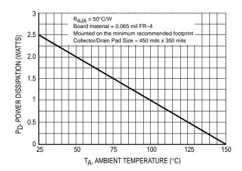
Figure 16. D<sup>2</sup>PAK Power Derating Curve
