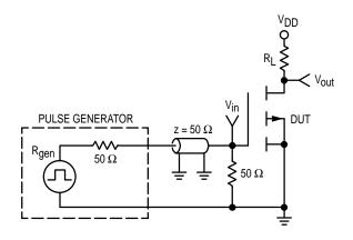
Figure 12. Switching Test Circuit
