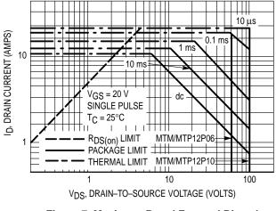
Figure 7. Maximum Rated Forward Biased Safe Operating Area
