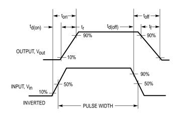
Figure 13. Switching Waveforms
