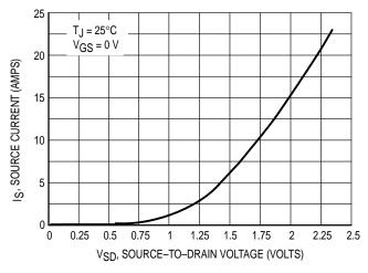
Figure 10. Diode Forward Voltage versus Current
