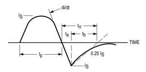
Figure 14. Diode Reverse Recovery Waveform
