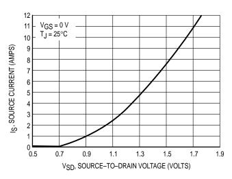
Figure 10. Diode Forward Voltage versus Current
