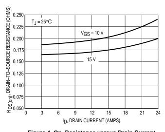
Figure 4. On–Resistance versus Drain Current and Gate Voltage
