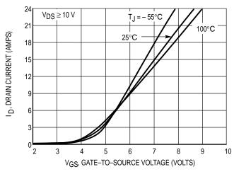
Figure 2. Transfer Characteristics
