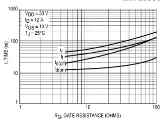
Figure 9. Resistive Switching Time Variation versus Gate Resistance
