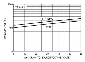
Figure 6. Drain-To-Source Leakage Current versus Voltage
