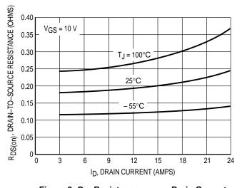
Figure 3. On–Resistance versus Drain Current and Temperature
