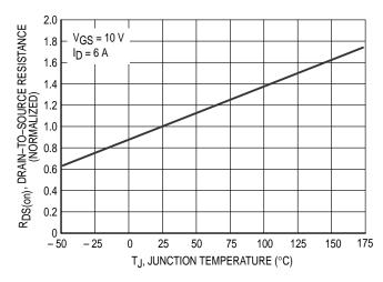
Figure 5. On–Resistance Variation with Temperature
