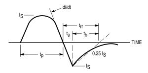
Figure 14. Diode Reverse Recovery Waveform
