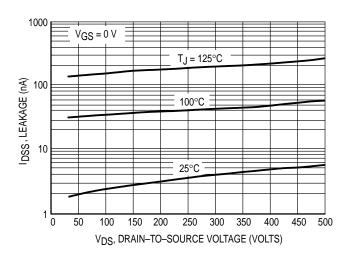
Figure 6. Drain-To-Source Leakage Current versus Voltage
