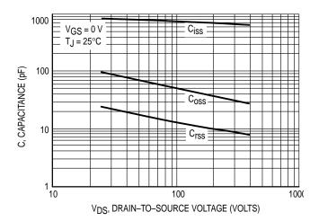
Figure 7b. High Voltage Capacitance Variation
