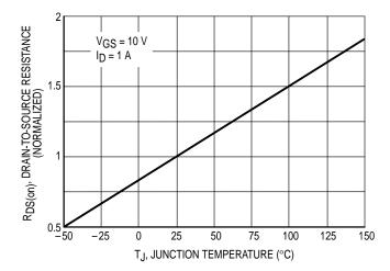
Figure 5. On–Resistance Variation with Temperature
