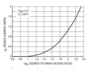
Figure 10. Diode Forward Voltage versus Current
