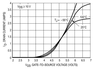
Figure 2. Transfer Characteristics
