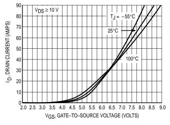
Figure 2. Transfer Characteristics
