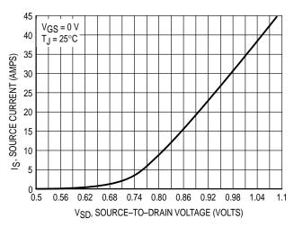
Figure 10. Diode Forward Voltage versus Current
