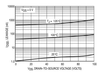
Figure 6. Drain-To-Source Leakage Current versus Voltage
