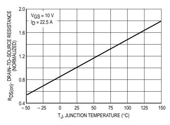
Figure 5. On–Resistance Variation with Temperature
