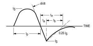
Figure 14. Diode Reverse Recovery Waveform
