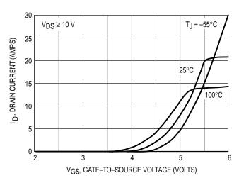
Figure 2. Transfer Characteristics
