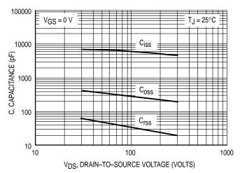
Figure 7b. High Voltage Capacitance Variation
