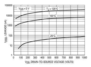
Figure 6. Drain-To-Source Leakage Current versus Voltage
