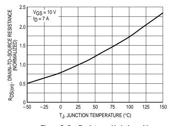
Figure 5. On–Resistance Variation with Temperature
