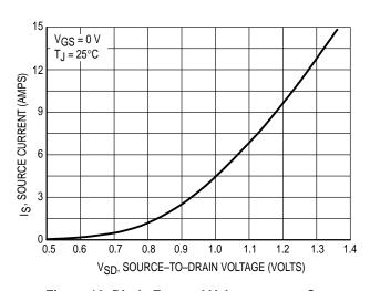
Figure 10. Diode Forward Voltage versus Current
