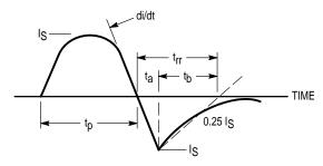
Figure 14. Diode Reverse Recovery Waveform
