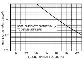
Figure 4. MTTF Factor versus Junction Temperature
