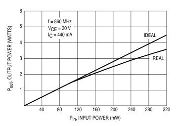
Figure 1. Power Output versus Power Input
