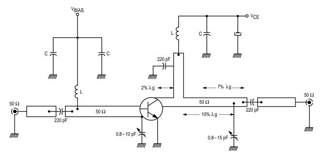
L=6 turns ID=1 mm Wire diameter=0.6 mm The lengths are given for f=860 MHz
