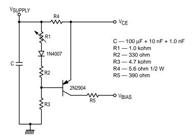
Figure 6. Class A Bias Circuit
