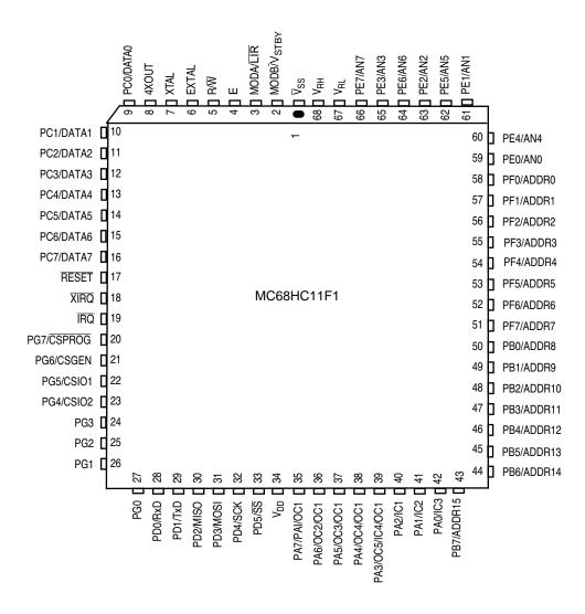
Figure 3 MC68HC11F1 68-Pin PLCC Pin Assignments
