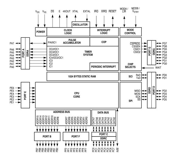
Figure 2 MC68HC11FC0 Block Diagram
