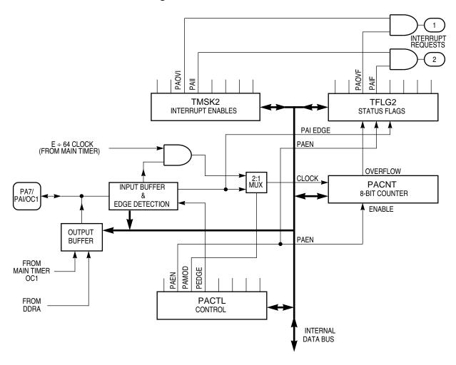
Figure 18 Pulse Accumulator Block Diagram
