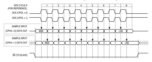
Figure 13 SPI Data Clock Timing Diagram
