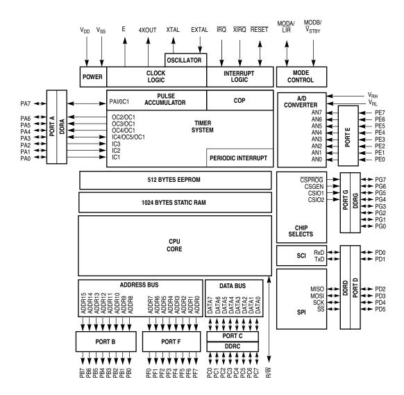
Figure 1 MC68HC11F1 Block Diagram
