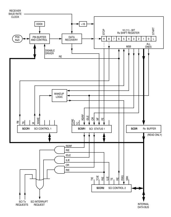
Figure 10 SCI Receiver Block Diagram
