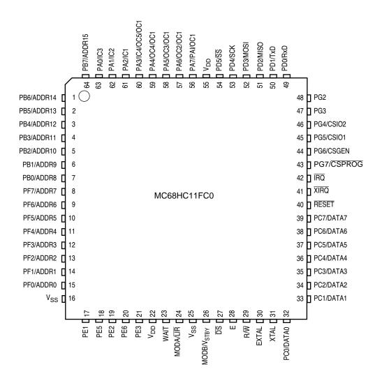
Figure 5 MC68HC11FC0 64-Pin QFP Pin Assignments
