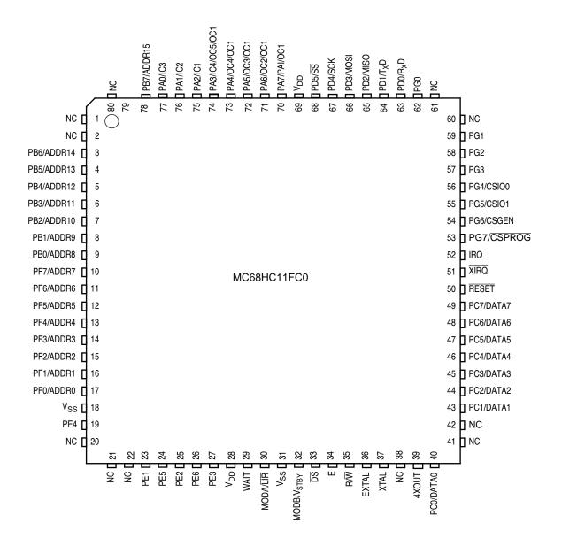
Figure 6 MC68HC11FC0 80-Pin TQFP Pin Assignments
