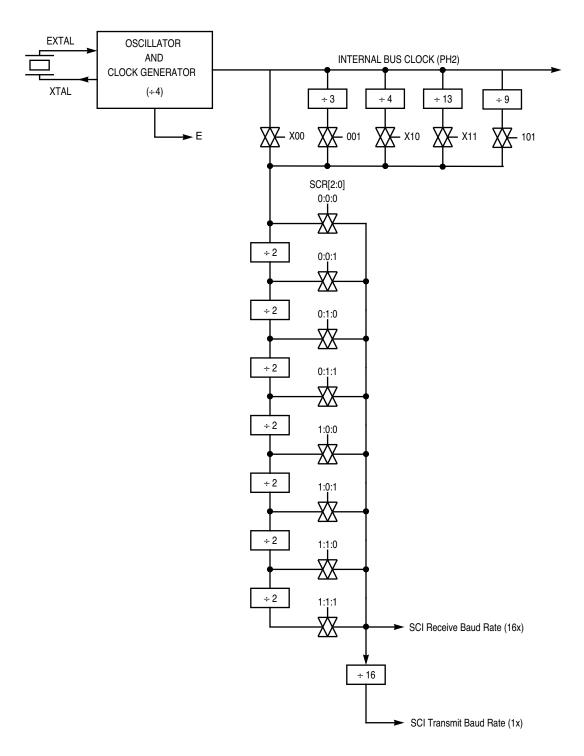
Figure 11 SCI Baud Rate Generator Block Diagram
