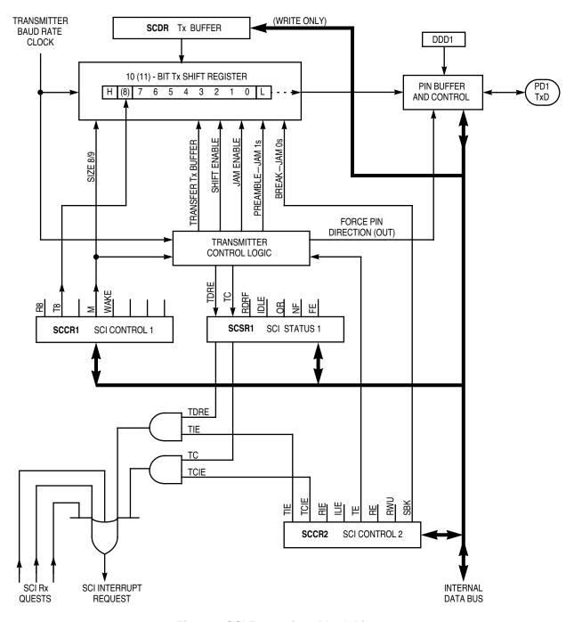
**Figure 9 SCI Transmitter Block Diagram**
