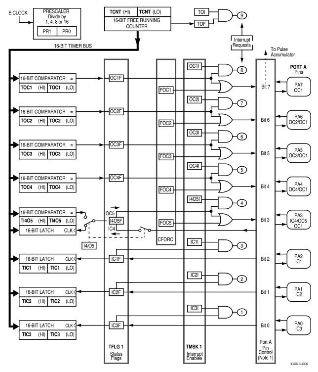
NOTE: Registers that control port A action include DDRA, OC1M, OC1D, PACTL, TCTL1 and TCTL2.
