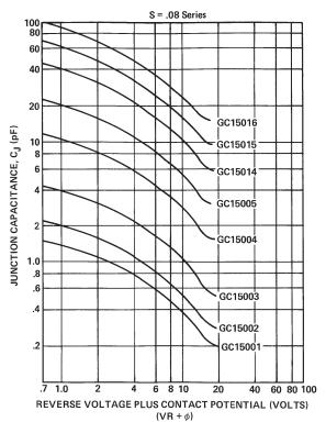
**Typical Capacitance vs Reverse Voltage**
