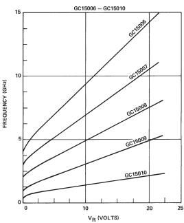
Frequency vs Reverse Voltage in Single Stage L-C Circuit
