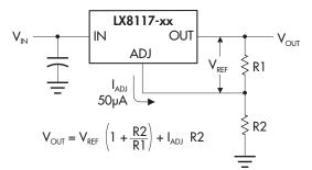
FIGURE 2 — BASIC ADJUSTABLE REGULATOR
