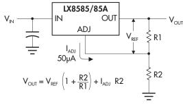
FIGURE 2 — BASIC ADJUSTABLE REGULATOR
