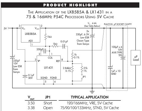
Thick traces represent high current traces which must be low resistance / low inductance traces in order to achieve good transient response.
