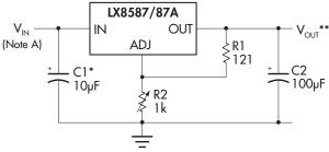
\* Needed if device is far from filter capacitors.
