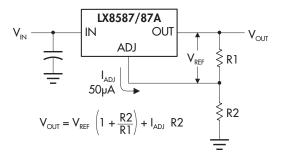
FIGURE 2 — Basic Adjustable Regulator
