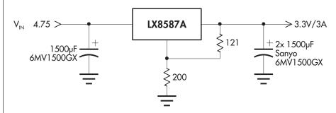
The output capacitors must be low ESR and low ESL type for good transient response.
