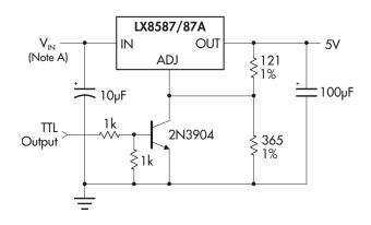
FIGURE 6 — 5V Regulator With Shutdown
