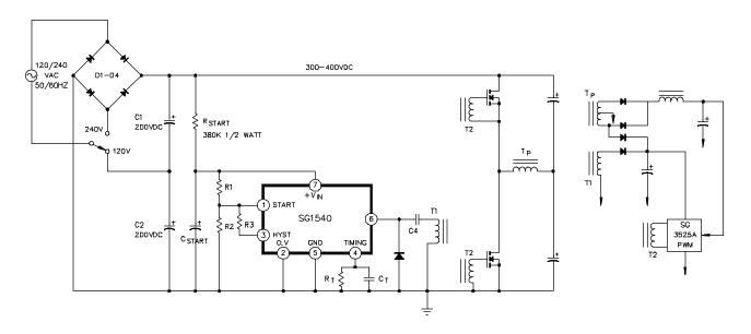
FIGURE 5 - SECONDARY-SIDE START-UP WITHOUT A LINE TRANSFORMER
