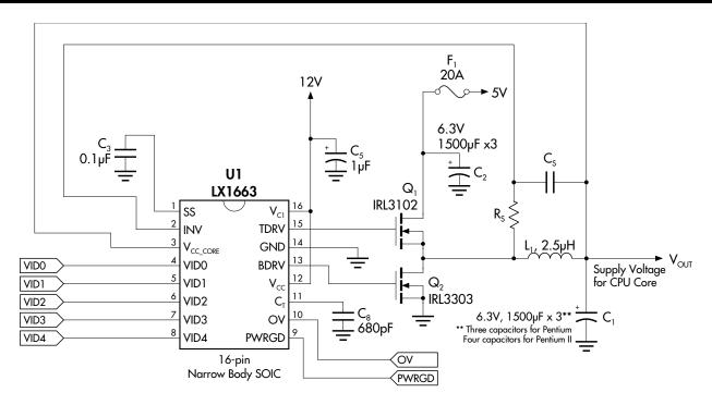
FIGURE 8 — Pentium II Processor Application With OVP, Power Good And Loss-Less Current Sensing (Synchronous)
