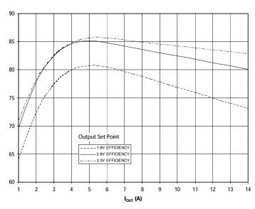
**FIGURE 4** — Efficiency Test Results: Synchronous Operation,  $V_{IN} = 12V$ .
