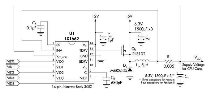
FIGURE 7 — LX1662 In A Non-Synchronous Pentium / Socket 7 Power Supply Application
