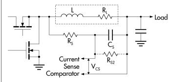
FIGURE 11 — Current Sense Circuit
