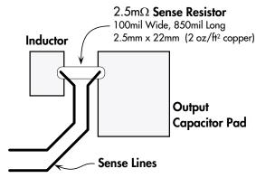
FIGURE 10 — Sense Resistor Construction Diagram
