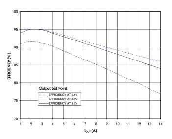
**FIGURE 3** — Efficiency Test Results: Synchronous Operation,  $V_{\rm IN} = 5V$
