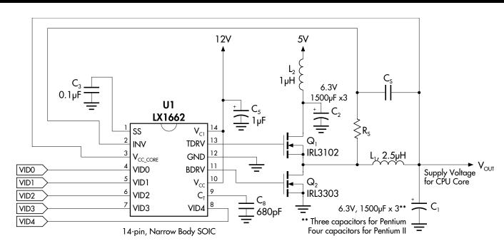
FIGURE 6 — LX1662 In A Pentium / Pentium II Processor Single Chip Power Supply Controller Solution With Loss-Less Current Sensing (Synchronous)
