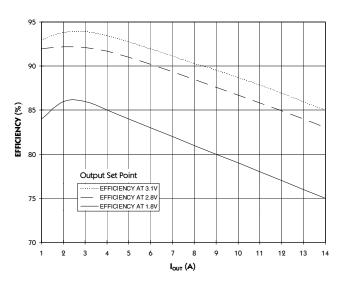
**FIGURE 2** — Efficiency Test Results: Non-Synchronous Operation,  $V_{IN} = 5V$
