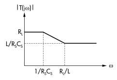
FIGURE 12 — Sensor Gain
