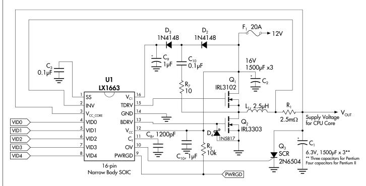
FIGURE 9 — Full-Featured Pentium II Processor Supply With 12V Power Input
