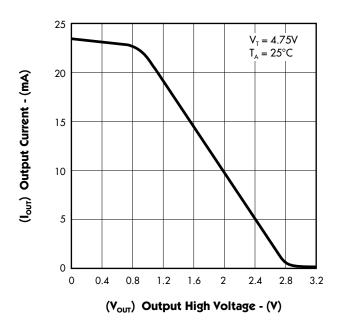
FIGURE 8. — OUTPUT CURRENT vs. OUTPUT HIGH VOLTAGE
