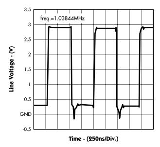
FIGURE 1B. — DRIVING WAVEFORM
