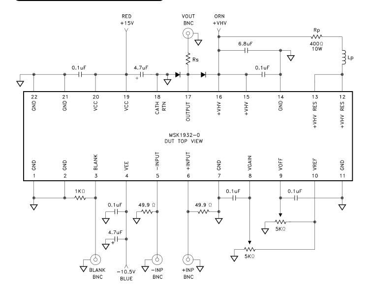
The connection circuit shown above is for the MSK 1932-0 evaluation board. The Rp and Lp are external components and must not be located near ground planes if possible. A high quality resistor such as Bradford Electronics P/N FP10-400 is required for optimum response times. Use an inductor with a high self-resonant frequency that can withstand the currents required for the application.
