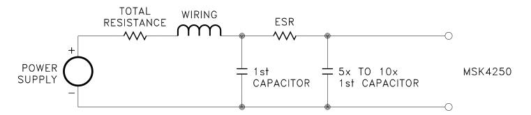
Be careful of the ripple current in all the capacitors. Excessive ripple current, beyond what the capacitors can handle, will destroy the capacitors.
