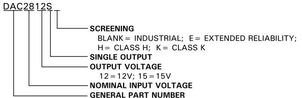
The above example is an industrial grade 12V single output converter
