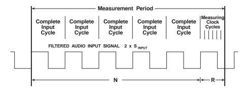
Figure 5: Measurement of an Rx Frequency
