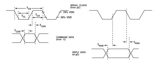
Figure 9: Timing Relationship for C-BUS Information Transfer
