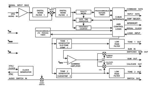
The MX803A is an audio signaling processor that provides inband tone signaling capabilities for LMR and other Radio systems. A low-power CMOS device, the MX803A is a member of the DBS800 (Digitally integrated Baseband Subsystem) IC family (See section 4.2). Supported Signaling systems include SelCall (CCIR, EEA, ZVEII, II, and III) 2-Tone SelCall and DTMF encode. The use of a non-predictive decoder and a versatile encoder, allows the MX803A to operate in any standard or non-standard tone system.
