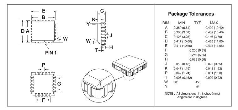
Figure 11: 24-pin PLCC Mechanical Outline: order as part no. MX803ALH
