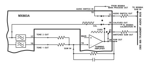
Figure 3: Example of Signal Switching in a DBS800 microcircuit
