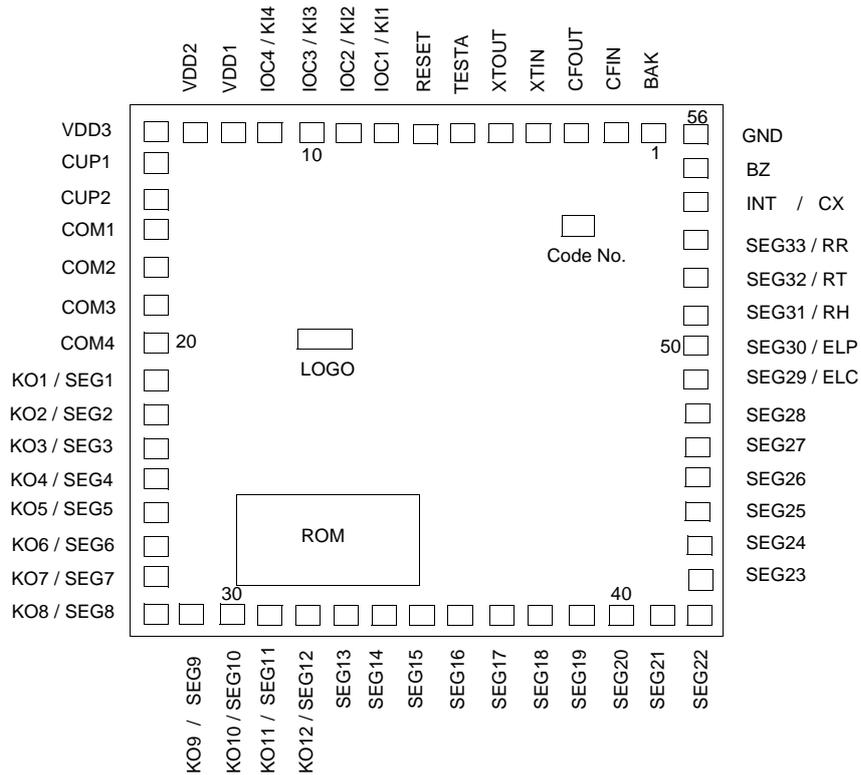
Note: The substrate of die must connect to GND.
