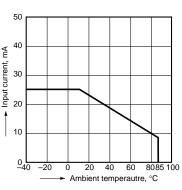
2. Load current vs. ambient temperature characteristics
