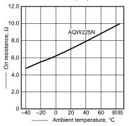
2.-(2) On resistance vs. ambient temperature characteristics
