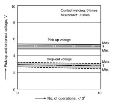
2-(2). Electrical life test (Lamp load) Tested sample: CM1aF-R-12V, 6 pcs. Load: 20A 13.5V DC Operate frequency: ON 1s, OFF 14s
