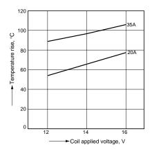
1-(2). Coil temperature rise (24V type) Tested sample: CM1F-24V, 4 pcs. Ambient temperature: 85°C 185°F Contact carrying current: 0 A, 15 A
