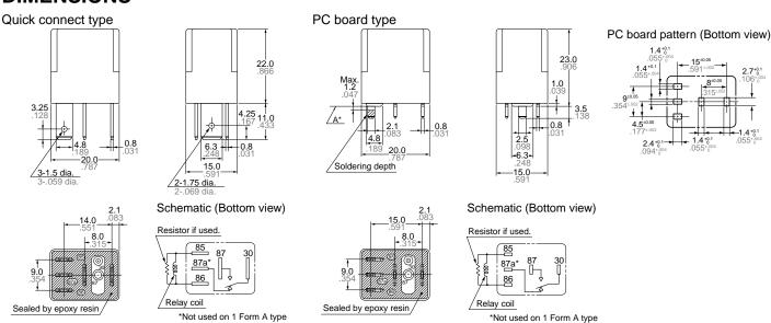
$\begin{array}{ll} \underline{\text{Dimension:}} & \underline{\text{General tolerance}} \\ \underline{\text{Max. 1mm.}} .039 \text{ inch:} & \pm 0.1 \pm .004 \\ 1 \text{ to 3mm.} .039 \text{ to .} 118 \text{ inch:} & \pm 0.2 \pm .008 \\ \end{array}$
