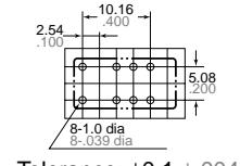
Tolerance:  $\pm 0.1 \pm .004$ Schematic (Bottom view)
