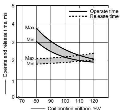
**6-(2). Operate/release time characteristics (without diode)**
