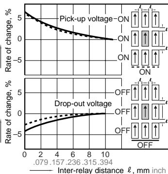
14. Actual load test (35 mA 48 V DC wire spring relay load)
