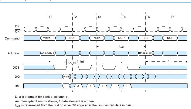
The Precharge command masks the last 2 data elements in the burst.
