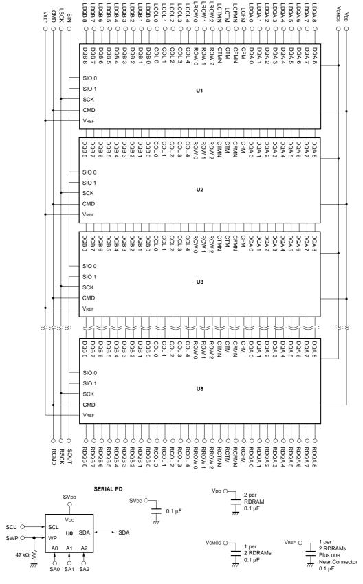
Remarks 1. Rambus Channel signals form a loop through the RIMM module, with the exception of the SIO chain.
