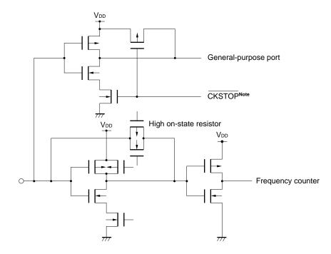
**Note** In this circuit, a current drained by noise does not increase even if the circuit is in the floating state, because of the internal signal being output when the clock stop instruction is executed.
