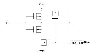
**Note** In this circuit, a current drained by noise does not increase even if the circuit is in the floating state, because of the internal signal being output when the clock stop instruction is executed.
