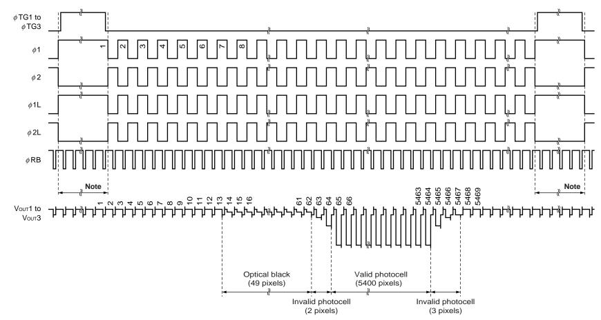
**Note** Input the  $\phi$  RB pulse continuously during this period, too.
