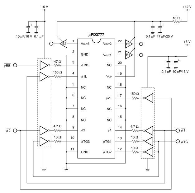
**Remark** The inverters shown in the above application circuit example are the 74HC04 (data rate < 2 MHz) or the 74AC04 (data rate: 2 to 4 MHz).
