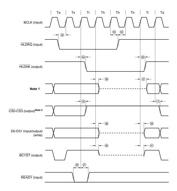
Notes 1. A2-A27 (output), BEO-BE3 (output), ST0-ST3 (output), R/W (output)
