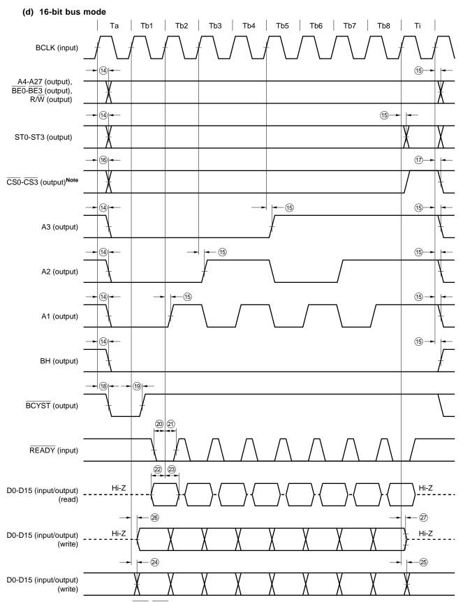
**Note** A28-A31 are output at  $\overline{CS0}$ - $\overline{CS3}$  when the chip select function is not used.
