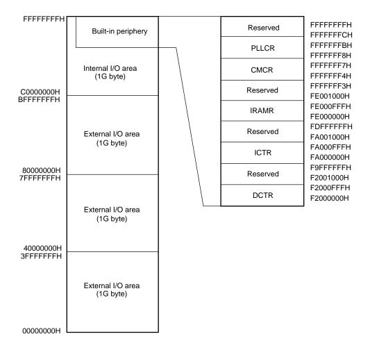
Figure 2-4. Internal I/O Area
