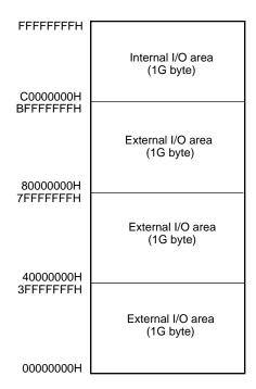
The cache function is not effective within the I/O space. When the chip select function is used, the area is used as the 256M-byte image space represented by A2-A27.
