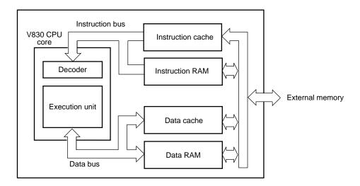
Figure 7-1. Built-In Cache Configuration
