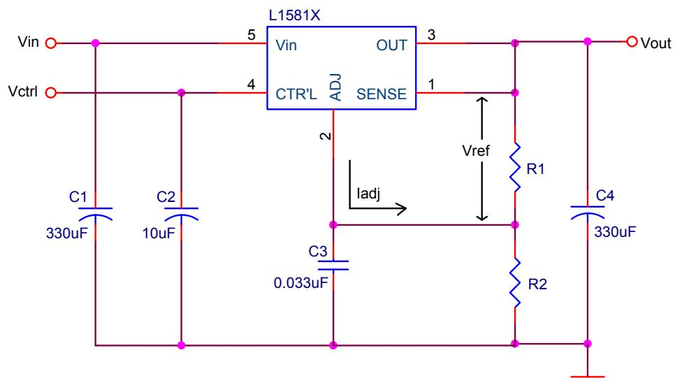
$$V_o = V_{ref} \left( 1 + \frac{R_2}{R_1} \right) + I_{adj} \times R_2$$
