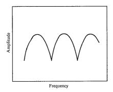
Fig. 5 Comb Type Filter Frequency Characteristic
