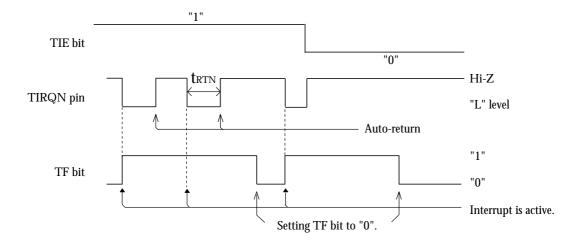
The auto-return time ( $t_{RTN}$ ), shown in the following figure and table, is determined by the source clock frequency set by register D in bank 1 bits FD3 and FD4.
