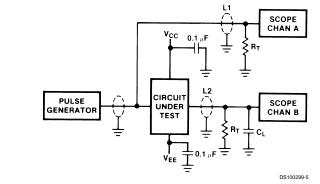
$\begin{array}{l} \mbox{Note:} V_{CC}, \ V_{CCA} = +2V, \ V_{EE} = -2.5V \\ \mbox{L1 and } L2 = equal length $50\Omega$ impedance lines \\ R_T = 50\Omega$ terminator internal to scope \\ \mbox{Decoupling } 0.1 \ \mu F from GND to V_{CC} and V_{EE} \\ \mbox{All unused outputs are loaded with $50\Omega$ to GND \\ \ C_L = Fixture and stray capacitance $\leq 3 \ pF \\ \end{array}$
