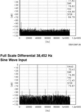
Half Scale Differential 1 kHz Sine Wave Input, f<sub>s</sub> = 153.6 kHz
