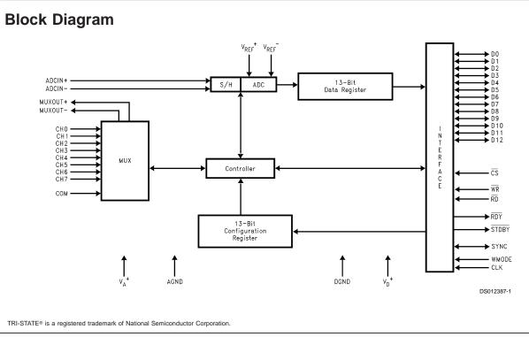
ADC12048 12-Bit Plus Sign 216 kHz 8-Channel Sampling Analog-to-Digital Converter
