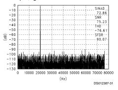
Half Scale Differential 75 kHz Sine Wave Input, fs = 153.6 kHz
