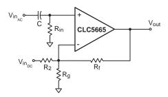
**Figure 5: Level Shifting Circuit**
