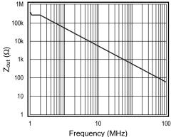
Figure 3: Equivalent Disabled Output Impedance
