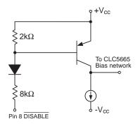
Figure 2: Pin 8 Equivalent Disable Circuit
