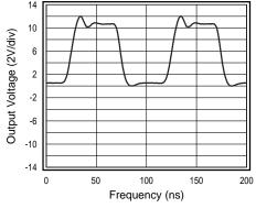
Figure 9: CCD Clock Driver
