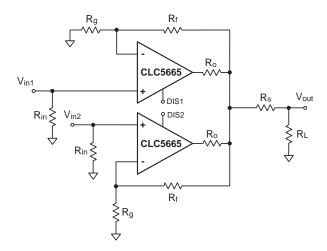
Figure 6: Output Connection for Multiplexing Circuits
