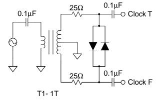
Figure 1: Method of Driving Clock Inputs
