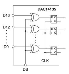
Figure 2: Digital Data Inputs with DS Input Pin
