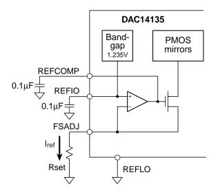
Figure 3: Internal Voltage Loop
