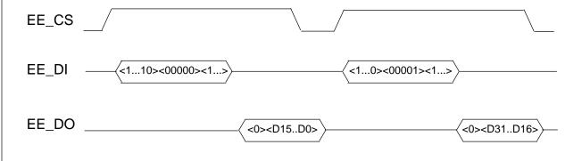
Figure 4. Serial EEPROM Access Protocol
