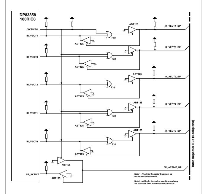
Figure 8. Inter Repeater Bus Connections
