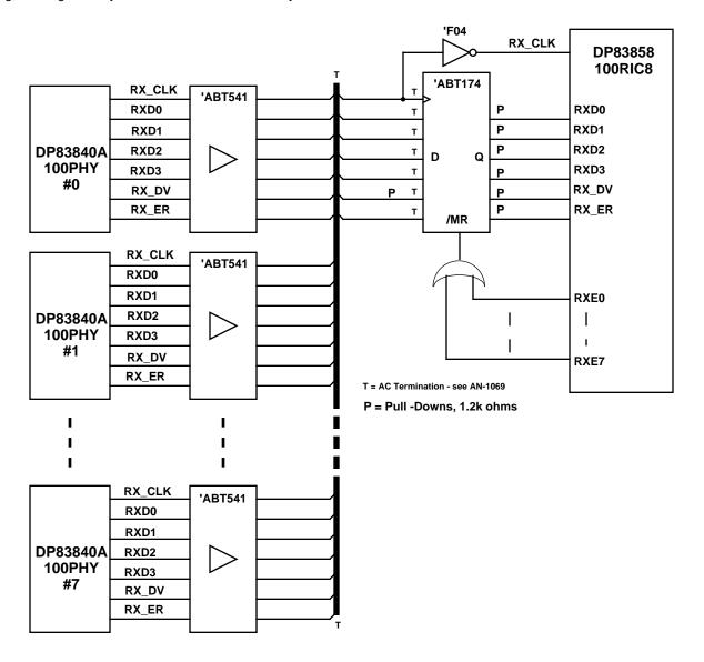
Figure 5. Recommended DP83840A to DP83858 Connections
