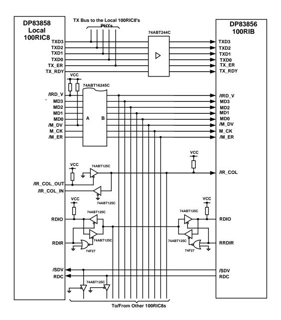
Figure 10. Typical DP83858 to DP83856 Connections
