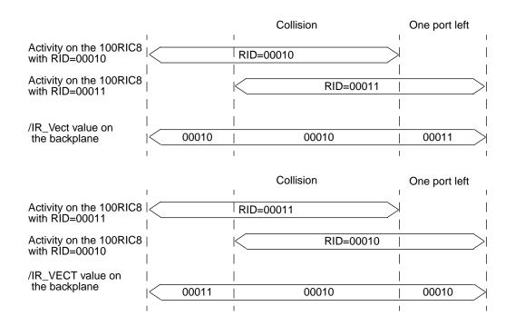
Figure 2. RID to /IR\_VECT Mapping
