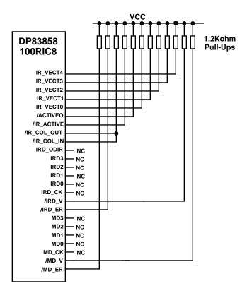
Figure 7. DP83858 Stand-alone Inter Repeater Bus Interface
