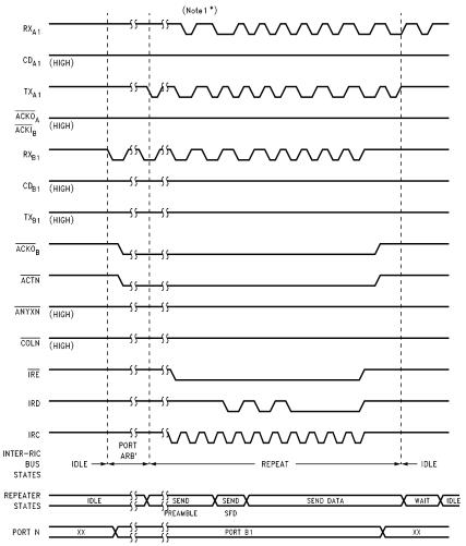
\*Note 1: The activity shown in RX<sub>A1</sub> represents the transmitted signal on TX<sub>A1</sub> after being looped back by the attached transceiver.
