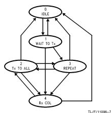
FIGURE 5.2. Inter-RIC Bus State Diagram
