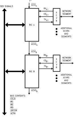
Note: In this example the Inter-RIC bus is configured to use active low signals.
