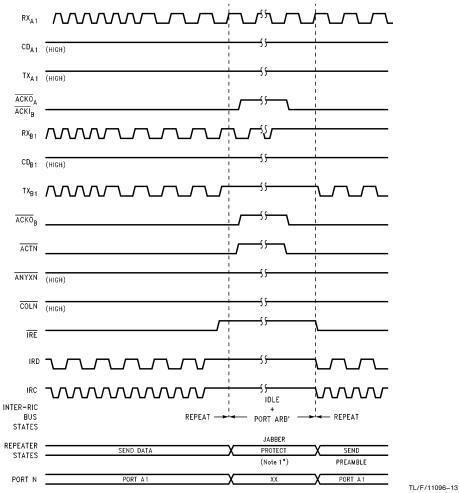
\*Note 1: The IEEE Specification does not have a jabber protect state defined in its main state diagram, this behaviour is defined in an additional MAU Jabber Lockup Protection state diagram.
