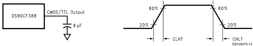
FIGURE 4. DS90CF388 (Receiver) CMOS/TTL Output Load and Transition Times
