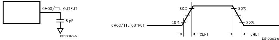
FIGURE 3. DS90CR288 (Receiver) CMOS/TTL Output Load and Transition Times
