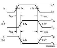
FIGURE 5. Driver Propagation Times
