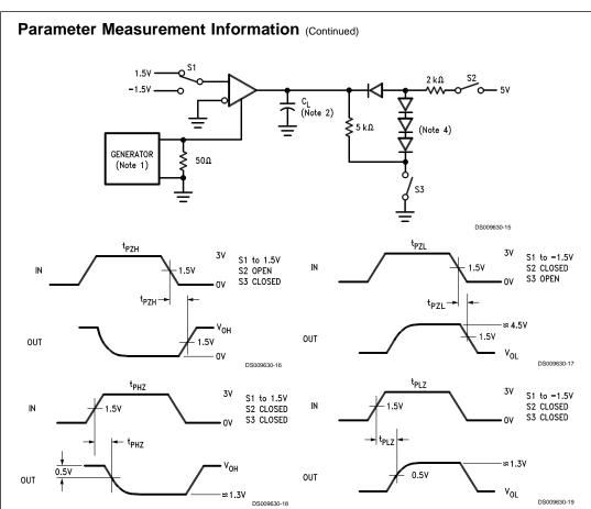
Note 11: The input pulse is supplied by a generator having the following characteristics: PRR = 1.0 MHz, 50% duty cycle,  $t_r \le 6.0$  ns,  $Z_O = 50\Omega$ .
