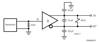
FIGURE 11. Typical Curve Driver Propagation Delay Test Circuit
