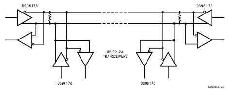
**Note:** The line length should be terminated at both ends of its characteristic impedance. Stub lengths off the main line should be kept as short as possible.
