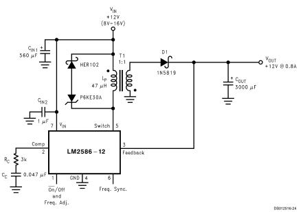
As shown in Figure 4, the LM2586 can be used as a flyback regulator by using a minimum number of external components. The switching waveforms of this regulator are shown in Figure 5. Typical Performance Characteristics observed during the operation of this circuit are shown in Figure 6.
