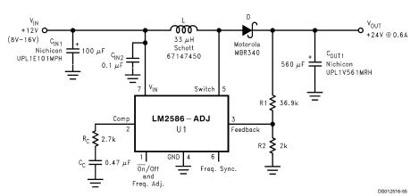
FIGURE 35. +12V to +24V Boost Regulator
