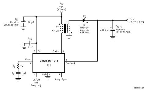
FIGURE 7. Single-Output Flyback Regulator
