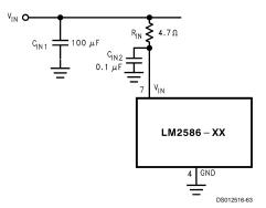
FIGURE 44. Input Line Filter
