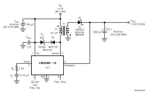
FIGURE 9. Single-Output Flyback Regulator
