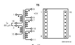
Top View FIGURE 23. Pulse PE-68413 (Surface Mount)
