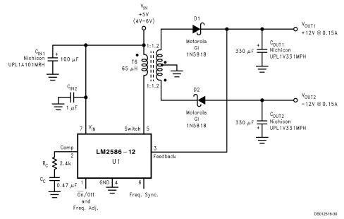
FIGURE 10. Dual-Output Flyback Regulator
