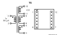
FIGURE 17. Coilcraft Q4437-B (Surface Mount)
