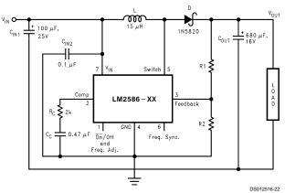
$C_{IN1}$  — 100 µF, 25V Aluminum Electrolytic  $C_{IN2}$  — 0.1 µF Ceramic L — 15 µH, Renco #RL-5472-5
