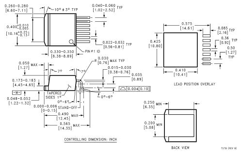
Order Number LM2586S-3.3, LM2586S-5.0, LM2586S-12 or LM2586S-ADJ Tape and Reel Order Number LM2586SX-3.3, LM2586SX-5.0, LM2586SX-12 or LM2586SX-ADJ NS Package Number TS7B
