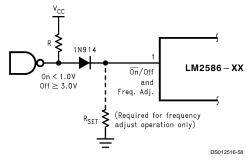
FIGURE 38. Shutdown Operation
