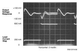
FIGURE 32.  $V_{\rm OUT}$  Response to Load Current Step
