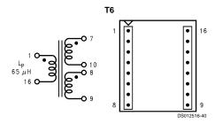
Top View FIGURE 22. Pulse PE-68414 (Surface Mount)
