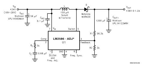
FIGURE 36. +24V to +36V Boost Regulator
