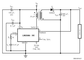
$C_{IN1}-100~\mu F, 25V$  Aluminum Electrolytic  $C_{IN2}-0.1~\mu F$  Ceramic  $T-22~\mu H, 1:1$  Schott #67141450 D-1N5820
