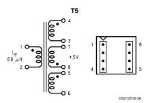
Top View FIGURE 18. Coilcraft Q4338-B
