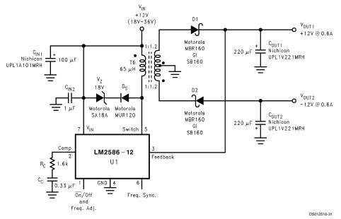
FIGURE 11. Dual-Output Flyback Regulator
