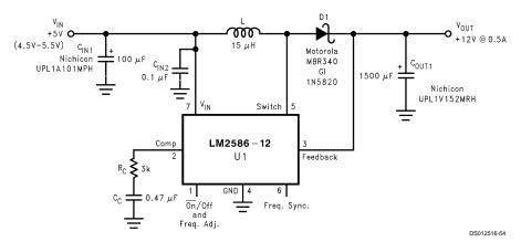
FIGURE 33. +5V to +12V Boost Regulator
