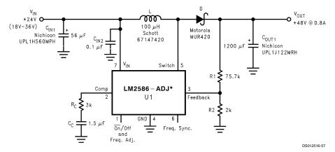
FIGURE 37. +24V to +48V Boost Regulator
