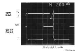
FIGURE 41. Waveforms of a Synchronized 12V Boost Regulator
