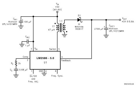
FIGURE 8. Single-Output Flyback Regulator
