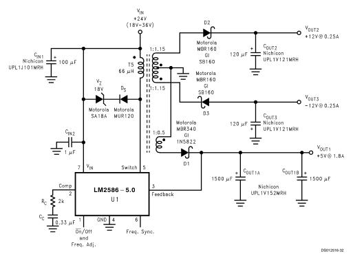
FIGURE 12. Triple-Output Flyback Regulator
