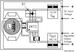
$C_{\mbox{\footnotesize{IN}}}$  - 15  $\mu\mbox{\footnotesize{F}},$  50V, Solid Tantalum Sprague, "594D series" C<sub>OUT</sub> - 68 μF, 16V, Solid Tantalum Sprague, "594D series" D1 - 1A, 40V Schottky Rectifier, Surface Mount
