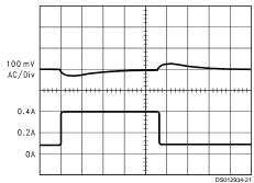
A: Output Voltage, 100 mV/div, AC-Coupled B: Load Current: 100 mA to 300 mA Load Pulse
