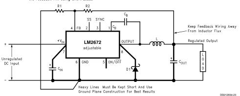
$C_{\mbox{\footnotesize{IN}}}$  - 22  $\mu\mbox{\footnotesize{F}},$  50V Tantalum, Sprague "199D Series"  $C_{\mbox{\scriptsize OUT}}$  - 47  $\mu\mbox{\scriptsize F},$  25V Tantalum, Sprague "595D Series"
