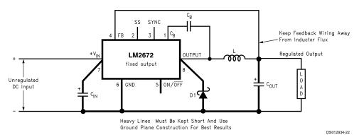
$C_{IN}$  - 22 μF, 50V Tantalum, Sprague "199D Series"  $C_{OUT}$  - 47 μF, 25V Tantalum, Sprague "595D Series" D1 - 3.3A, 50V Schottky Rectifier, IR 30WQ05F L1 - 68 μH Sumida #RCR110D-680L
